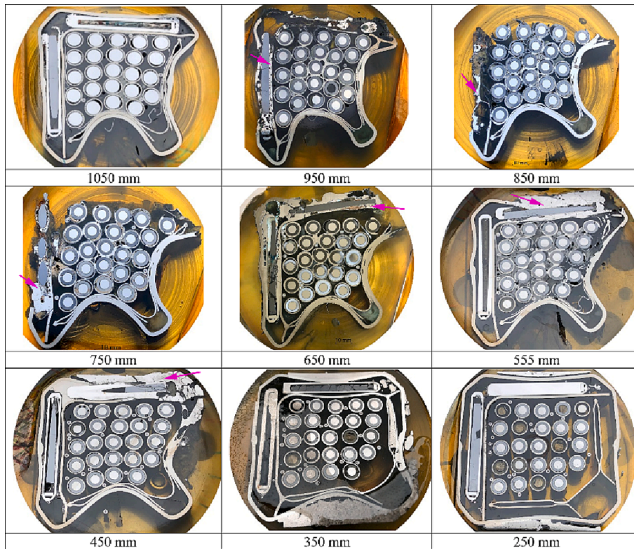
Fig. 12. Bundle cross sections at different elevations (arrows show regions with eutectic absorber melt).
