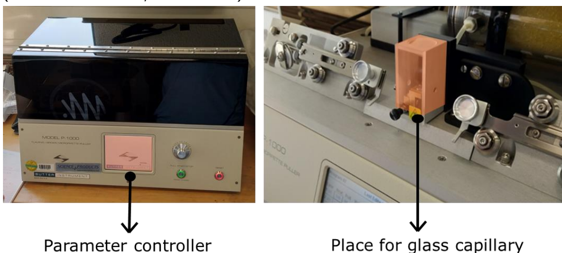
Figure A. 1: P-1000 micropipette puller system. (Setup at glass workshop INT)
