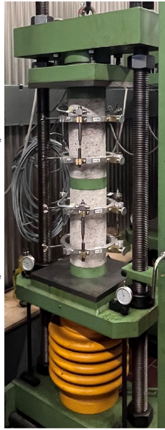
FIGURE 1 Experimental creep setup used in this study.
