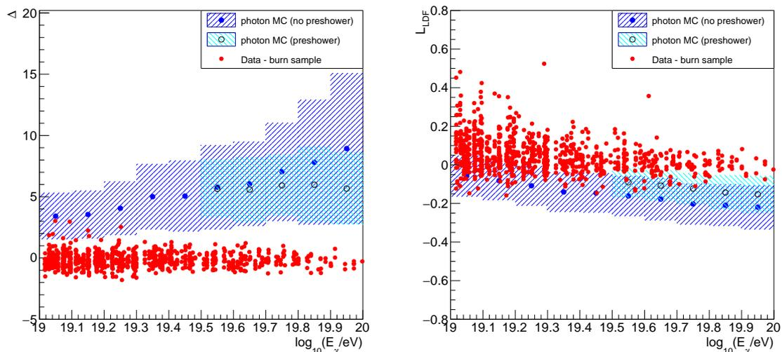
**Figure 4.** Distribution of  $\Delta$  (left) and  $L_{\text{LDF}}$  (right) as a function of the photon energy  $E_\gamma$  for the burn sample and photon simulations. Preshowering photons are shown only in the energy range in which they represent a fraction of the selected events larger than 3%. The bands represent one standard deviation of the photon distributions.
