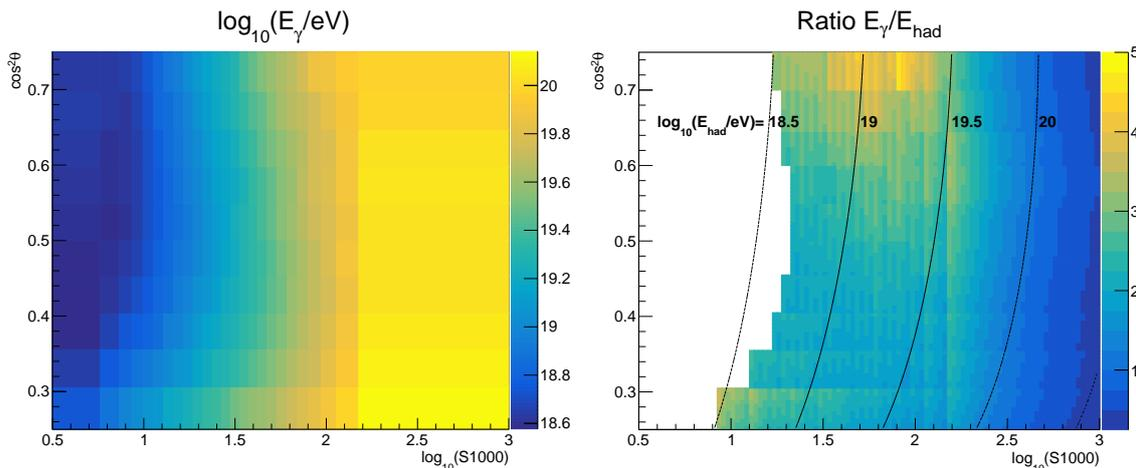
**Figure 3.** Look-up table used to assign the photon energy  $E_\gamma$  (left) and ratio of  $E_\gamma$  to the energy  $E_{\text{had}}$  calibrated with data and representing the correct scale for nuclear primaries (right). The ratio is shown only for  $E_\gamma > 10$  EeV, corresponding to the range studied in this work. The lines in black show the contours corresponding to four values of  $E_{\text{had}}$  to facilitate the comparison of the energy scales.
