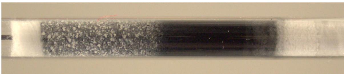
**Figure S5** A photograph of the catalyst bed after the reaction.
