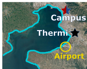
Figure 3.9.: Map with marked wind sensors on the Campus, in Thermi (KEΔEK) and at the airport. Wind speed as well as wind direction are important parameters for the up- and downwind setup. The map is a cut version of Figure 3.1 and depicts the wind sensors as stars. In an adapted form, small maps will be used throughout this work to illustrate measurement alignments and corresponding wind conditions.
