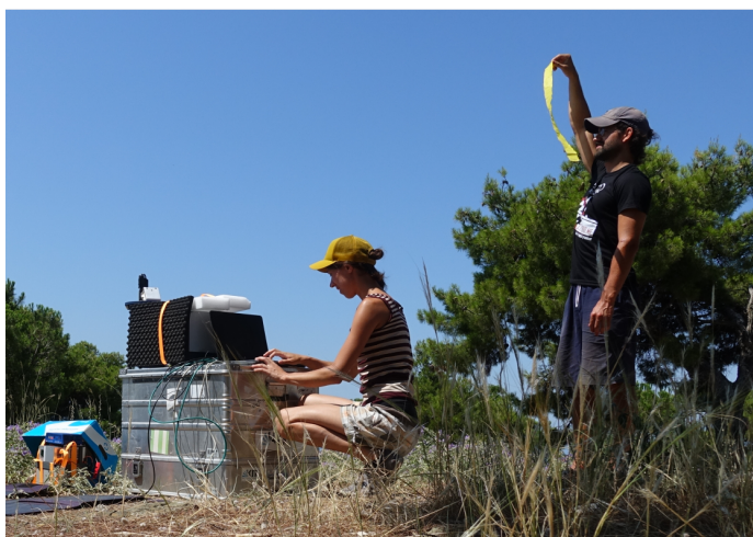
Figure 3.11.: Usage of a kite for the estimation of the wind direction (Photo taken at the measurement site in the Seych Sou park in July 2022 with a private digital camera and self-timer).
