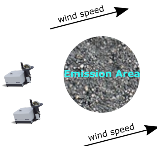
Figure 3.4.: Sketch of the background measurement setup (EM27/SUN images from https://www.bruker.com , December 2022)
