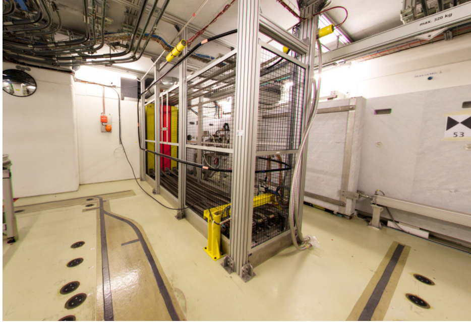
Figure 5.12: Photo of the CHARM target room with the movable shielding walls retracted [104].
