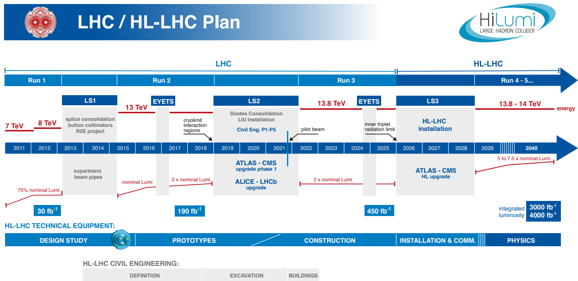
Figure 1.2: Current LHC baseline plan for the next decade and beyond, showing the collision energy (upper line) and luminosity (lower line) [5].
