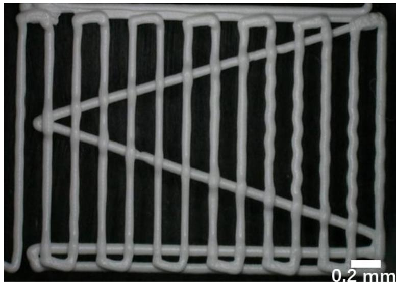
**Fig. 5.1.4.5** V-shaped test structure for determination of the critical span distance, i.e. the span up to which no significant deformation or breakage is observed by visual inspection, exemplarily shown for filaments printed from the paraffin oil-based ink. The composition of all inks used in these printing experiments is given in Table 3.3.1.
