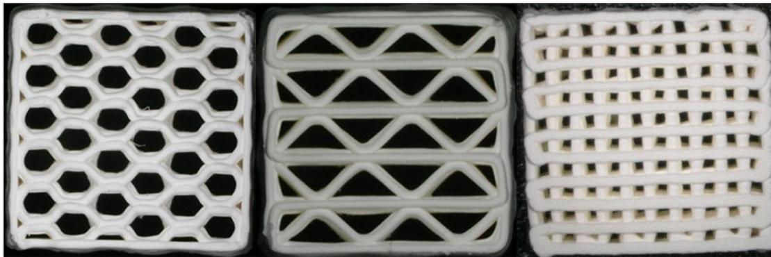
**Fig. 5.1.3.2** Macromorphology of sintered honeycomb, triangular and log-pile structures printed with the PDMS-based ink described in Table 3.3.1.
