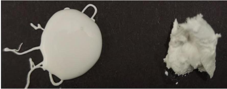
**Fig.5.1.2.1** Droplets of the suspension based on LLZTO particles and PDMS as bulk phase (left), and with ethylene glycol as second fluid phase (right).
