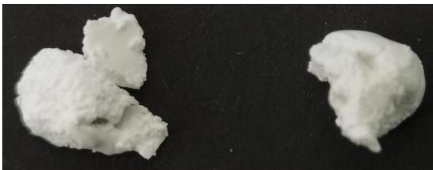
**Fig.5.1.2.3** Droplets of the suspension based on LLZTO particles and castor oil as bulk phase (left), and with non-ionic surfactant Span 80 (right).
