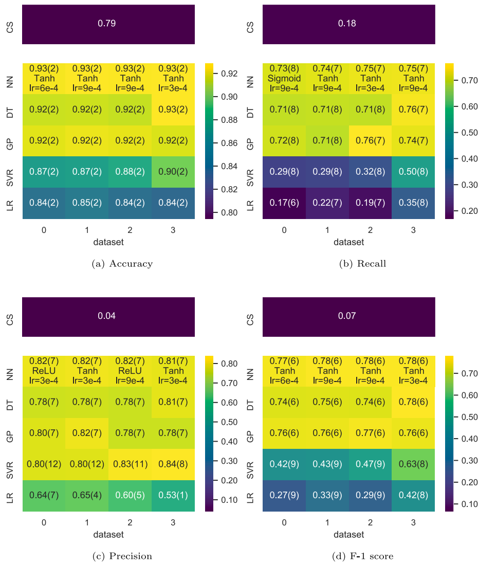
Fig. 7. Model and dataset comparison for confusion matrix results Accuracy, Recall, Precision and F1-score. Neural Net, Decision Tree, and Gaussian Processes show the overall best results for correctly predicting if the collector should be cleaned or not. The metrics for the current cleaning schedule (CS) are included for comparison.
