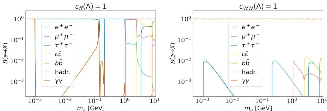
**Figure 1.** Branching ratios for ALP decays  $a \rightarrow X$  in the  $c_{ff}$  scenario (left) and the  $c_{WW}$  scenario (right). The ALP couplings are fixed to  $c_{ff}(\Lambda) = 1$  and  $c_{WW}(\Lambda) = 1$  at the cutoff scale  $\Lambda = 4\pi$  TeV.
