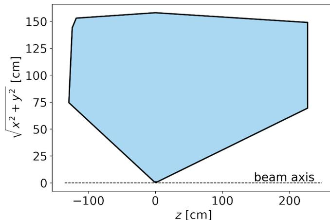
**Figure 9.** Schematic drawing of the Belle II detector used to select invisible ALP decays. The displayed geometry includes the central drift chamber and the calorimeter, as specified in the text. The detector is assumed to be symmetric around the beam axis  $z$ .
