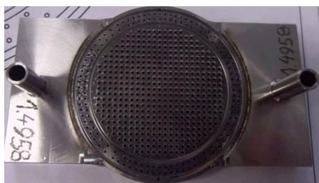
Figure 4. Assembled burner plate with laser-welded adapters.
