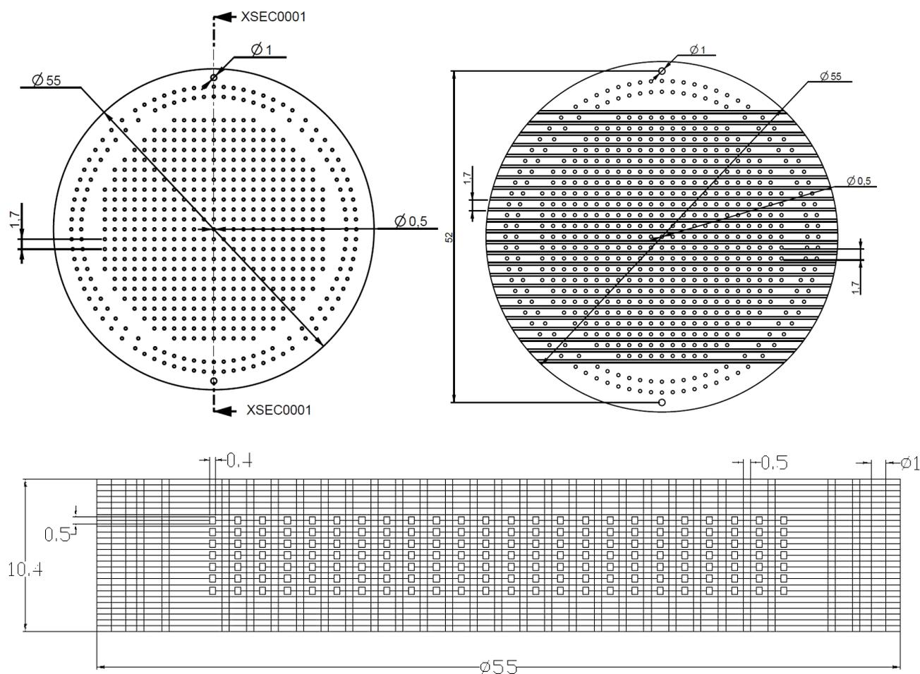
**Figure 1.** CAD of the burner plate. Top left: Top view including double circled cover gas nozzles. Top right: Design of layers with cooling channels. Bottom: Cross-section.
