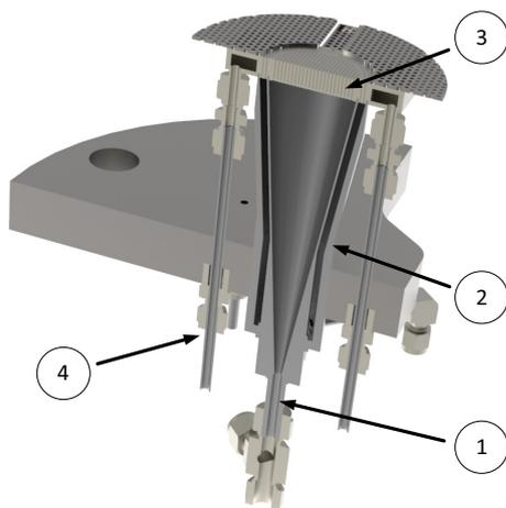
Figure 5. Sectional drawing of the burner unit, including a static mixer (1), diffuser (2), burner plate (3), and thermal oil circuit (4).
