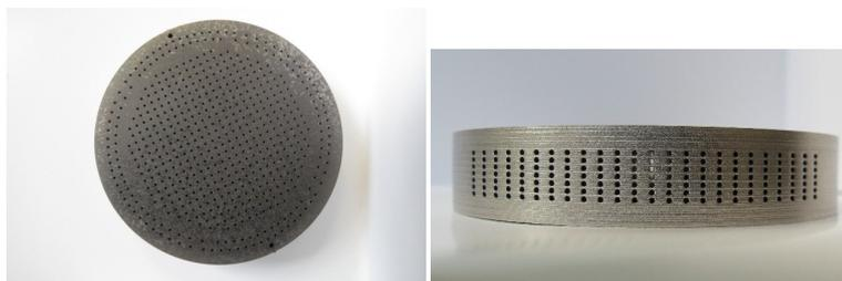
Figure 3. Burner plate after diffusion bonding.
