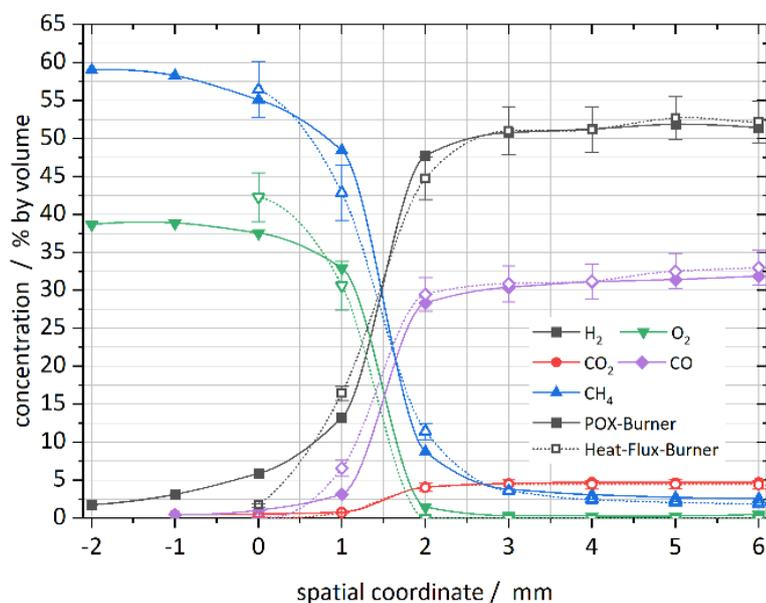
**Figure 6.** Comparison of the major combustion species profiles of CH<sub>4</sub>/O<sub>2</sub> flames ( $\phi = 2.7$ ,  $T_p = 300$  K,  $p = 1$  bar<sub>a</sub>) on the HFB and the POX burner, measured by invasive sampling and analyzed by gas chromatography (full symbols: POX burner, empty symbols: HFB).
