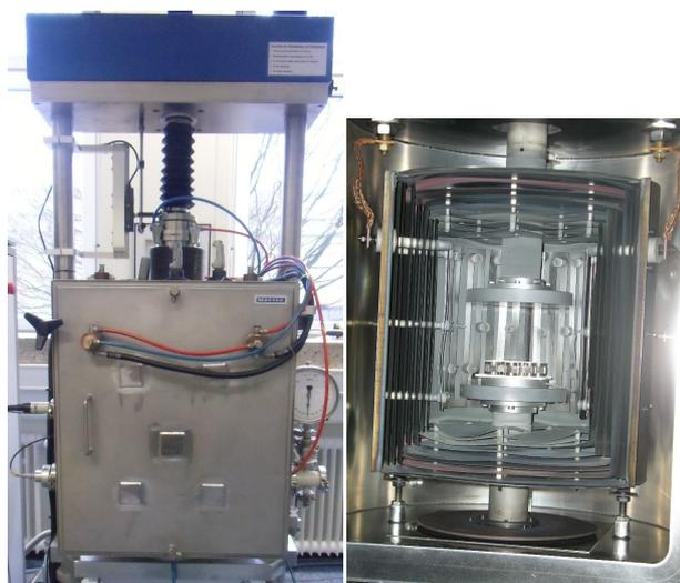
**Figure 2.** 20-kN diffusion bonding furnace.
