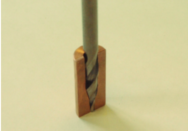
Fig. A.27: Photo of driller and cut of the manufactured Potter horn.
