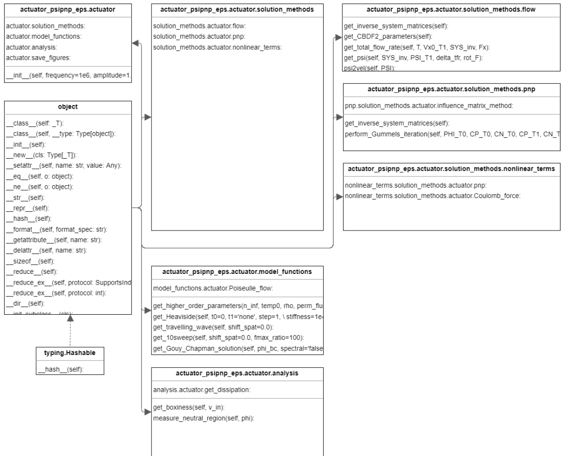
Figure C.1: UML diagram of the solver displaying selected classes and sub-classes.
