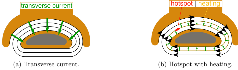
Figure 3.30.: Illustration of current paths in the dry wound, non-insulated VR coil for an existing hotspot. The superconductor and its current are shown as a spiral with a current direction. A transverse current flow skips this spiral, can redistribute, and therefore cause local heating. Copper and iron bodies are sketched in solid colors and are not so scale.
