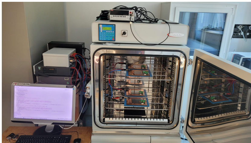
Figure A.12.: Climatic chamber setup used to study the humidity sensitivity of sensors. The sensors (four 2S sensors) are mounted on long-term boards and placed inside the chamber. Measurement devices located next to the chamber allow to measure leakage currents while the sensors are exposed to different relative humidity levels.
