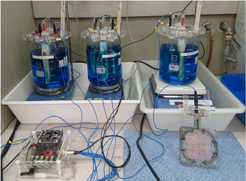
**Figure 2.14:** Cu electroplating setup to perform the copper deposition on 6 substrates in parallel. (Figure reproduced from [121])
