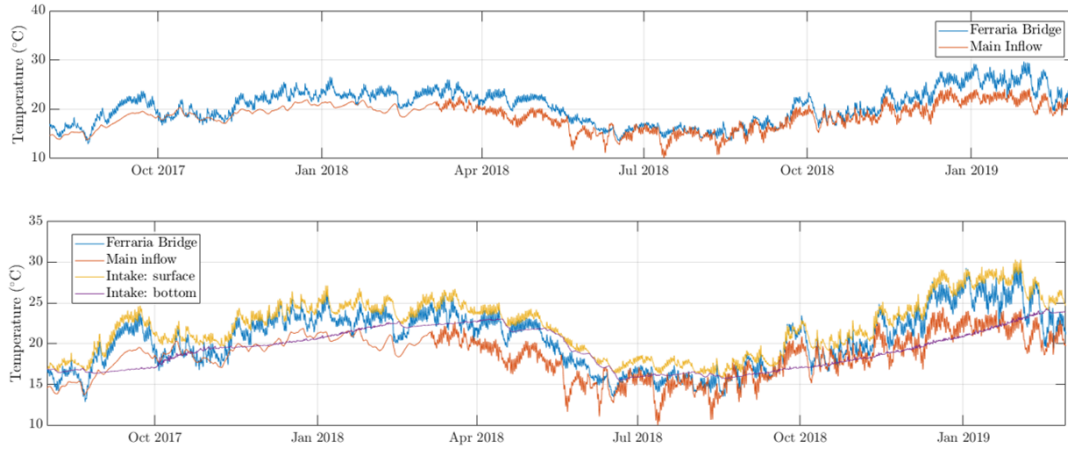
Figure A.8.: Analysis of possible density currents based on simulated temperatures at the Inflow, Ferraria Bridge and at the Intake for the whole simulation period. Top: comparison of the temperatures at the Ferraria Bridge and the main Inflow. Bottom: comparison of the three relevant locations.
