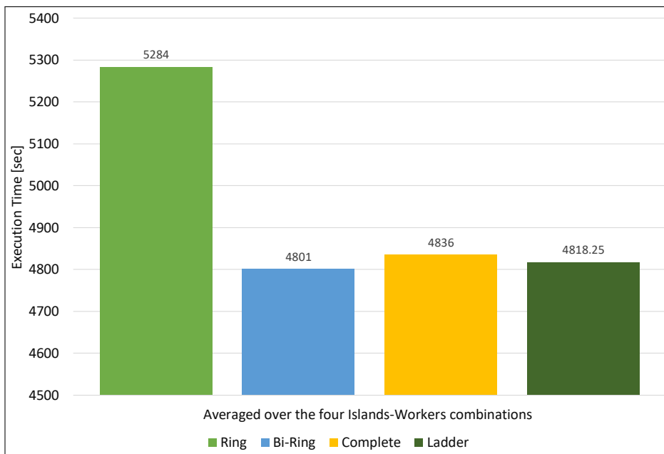
Figure 5.23.: Execution time of the Coarse-Grained - Global Hybrid Model for each communication topology averaged over the four applied islands-workers combinations
