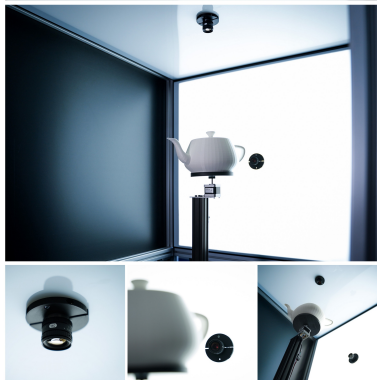
Figure 1: These are pictures of our HALODOME-setup which ought to simulate inline inspection of manufactured pieces.
