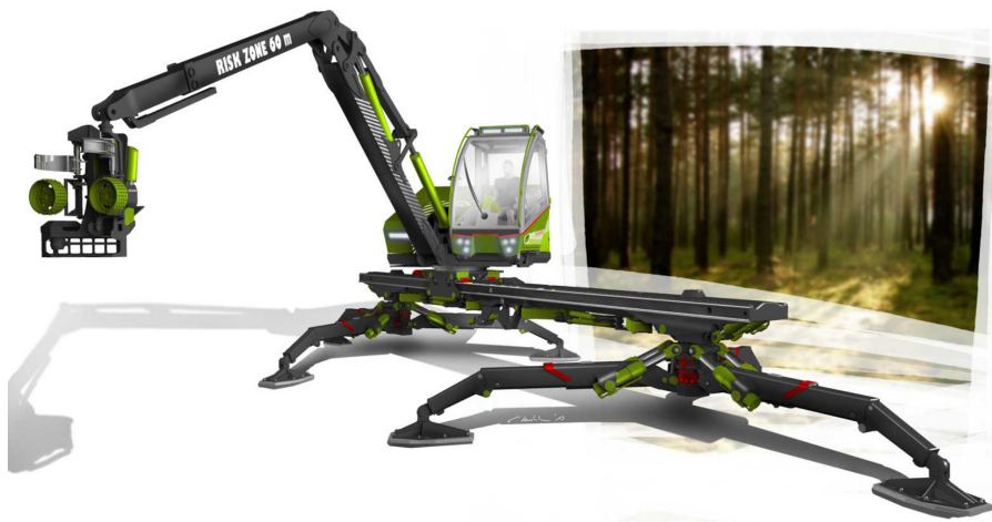
Figure 1: Rendering of the Portal Advancing Mechanism with a forestry crane [15]
