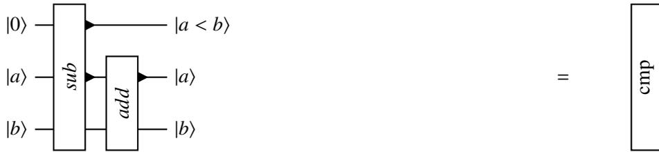
**Figure 2.16** In-place comparison circuit using QFT addition and subtraction. The comparison uses the fact that the subtraction results in  $2^{n+1} - b + a$  effectively setting the most significant bit if  $a$  is smaller than  $b$ .
