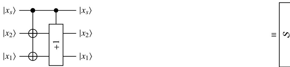
**Figure 5.2** The circuit converts a quantum state of a two's complement number to a state of an unsigned number by flipping all bits condition on the sign bit and adding one.
