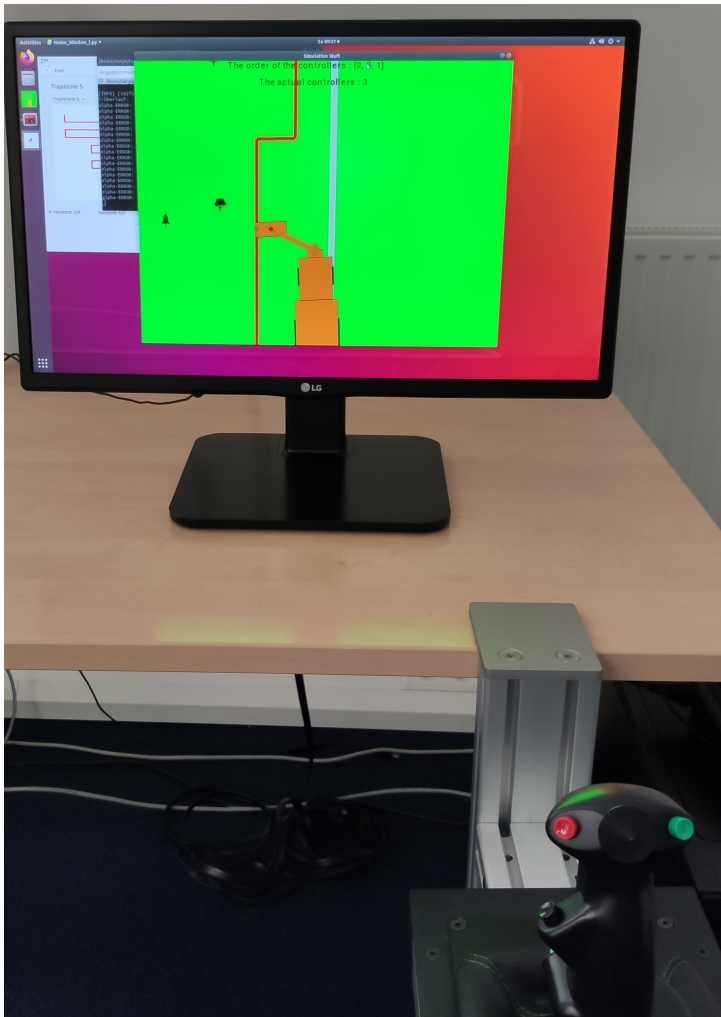
Figure 6.3: Graphical User Interface of the scenario with the vehicle manipulator in the first experiment. The manipulator reference (red line) was used only by FISC and for the evaluation. LISC and NCC do not require the manipulator reference [VIH22]. ©2022 IEEE
