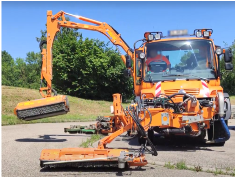
Figure 1.1: An exemplary image of a large vehicle manipulator with three working attachments.
