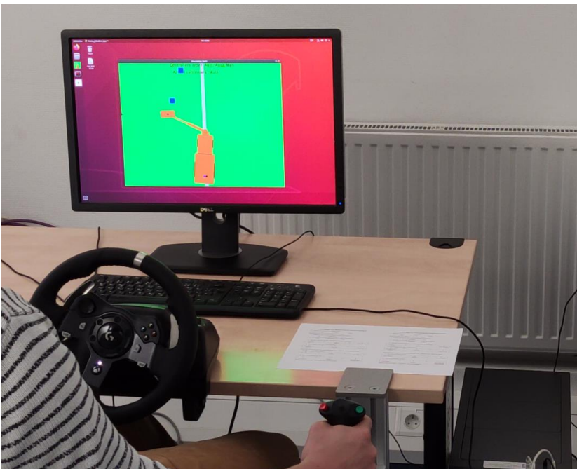
Figure 6.1: Picture of the test bench showing the vehicle manipulator. The GUI on this image belongs to the second experiment, see Section 6.3 [VRH22]. ©2022 IEEE
