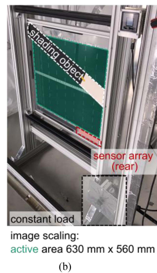
Fig. 3. (a) Sketched setup in our shading experiment to measure the magnetic flux density \vec{B} by MFI. The close-up view is meant to illustrate the principal correlation between the current density in the solar module and the resulting magnetic flux density and is not to scale. The solar module is illuminated from the front while the MFI is done from the rear. During the experiments, the operation point of the solar module is adjusted by a constant load between 0 \Omega and 10 \Omega . (b) Image of the setup in the solar simulator. The area covered with solar cells (highlighted green) is 630 \text{ mm} \times 560 \text{ mm} . The sensor array (highlighted red) is visible through the transparent back sheet.
