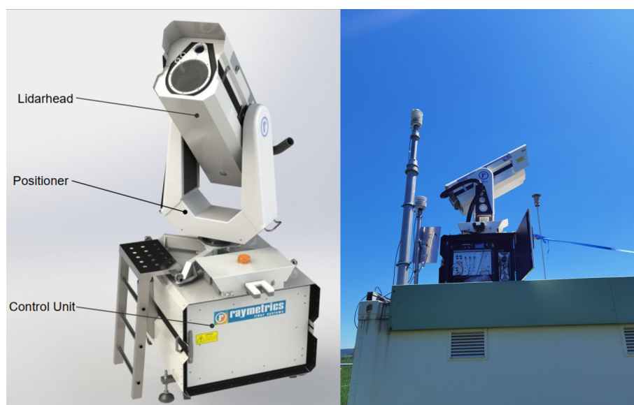
Figure 2.1: The picture of KASCAL (left, provided by Raymetrics Inc.) and the photo of the lidar on the roof of a mobile container taken during the Swabian MOSES campaign in July 2021 (right, photo by Hengheng Zhang).
