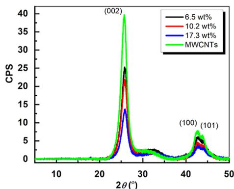
**Figure 1.** XRD patterns for the MoS<sub>x</sub>@MWCNTs indicating their amorphous nature, different loadings of MoS<sub>x</sub> wt % are indicated in the legend.
