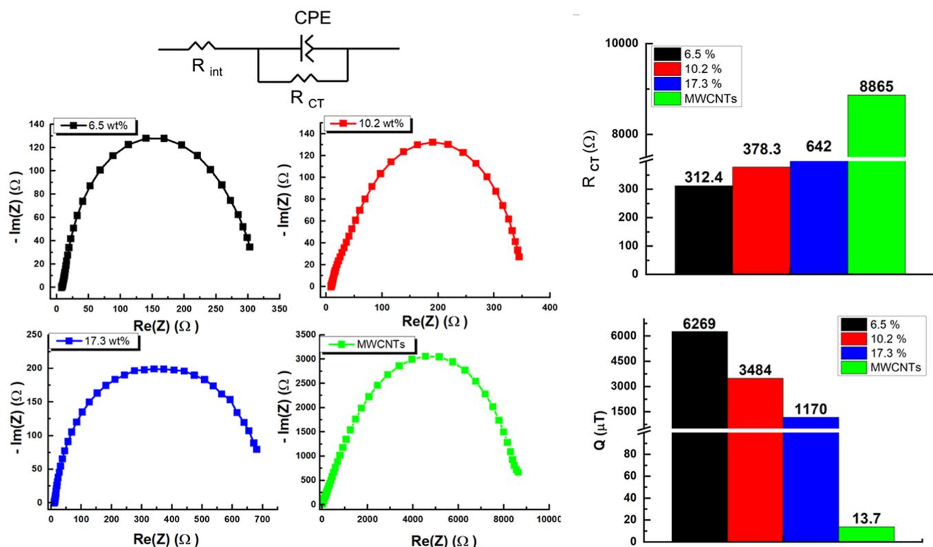
Figure 10. EIS profiles for the different materials (MWCNTs and different loadings of  $MoS_x@MWCNTs$ ) showing the notable trends of decreasing capacitance and increasing charge-transfer resistance upon increasing the  $MoS_x$  wt % in the composite (bar charts).
