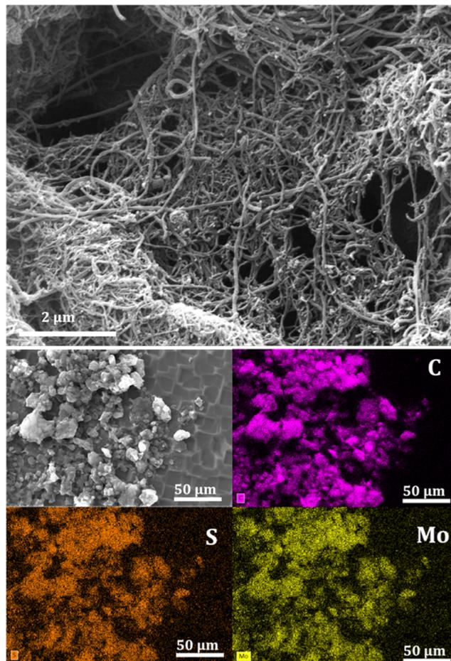
**Figure 2.** SEM image of the MoS<sub>x</sub>@MWCNTs showing no evidence for the formation of agglomerates or particulates of MoS<sub>x</sub> outside the MWCNT matrix and the EDX maps (imaged at lower magnification for clarity) showing excellent tracing of the elemental (C, S, and Mo) maps to that of the SEM image.
