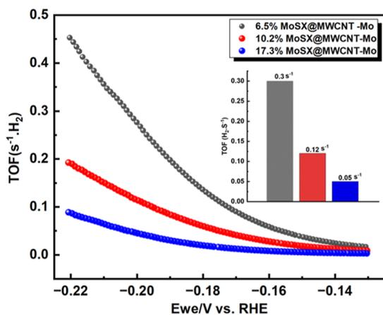
**Figure 9.** TOF for the three catalysts of MoS<sub>x</sub>@MWCNTs with increasing MoS<sub>x</sub> wt % at different applied bias values; the inset shows the TOF for the three catalysts at an overpotential of 200 mV vs RHE, values calculated based on Mo sites.
