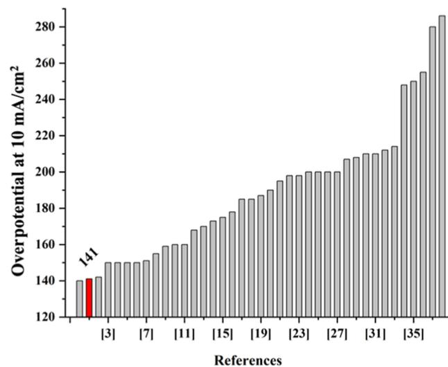
**Figure 8.** Plot of overpotentials reported to derive a current density of 10 mA/cm<sup>2</sup> from different MoS<sub>2</sub> HER catalysts, the result of the current study is highlighted, and references are reported in the Supporting Information.
