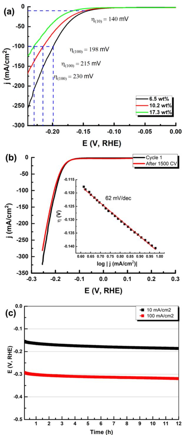
**Figure 7.** (a) LSV scans of the different MoS<sub>2</sub> loading on MWCNTs and that of MWCNTs, (b) LSV scans for the 6.5 wt % of MoS<sub>2</sub>@MWCNTs showing its stability after extended cycles and in inset of the corresponding Tafel plot, and (c) CP plot for the 6.5 wt % of MoS<sub>2</sub>@MWCNTs indicating its extended stability at two different current density values. All measurements were conducted in the 0.5 M H<sub>2</sub>SO<sub>4</sub> solution.
