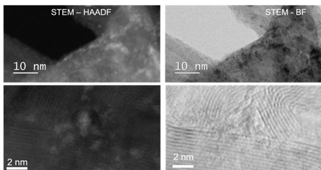
**Figure 3.** STEM-HAADF and BF images of the  $\text{MoS}_x$ @MWCNTs showing the nanoparticles of  $\text{MoS}_x$  coating the MWCNTs (bright spots in the HAADF and dark spots in the BF images).
