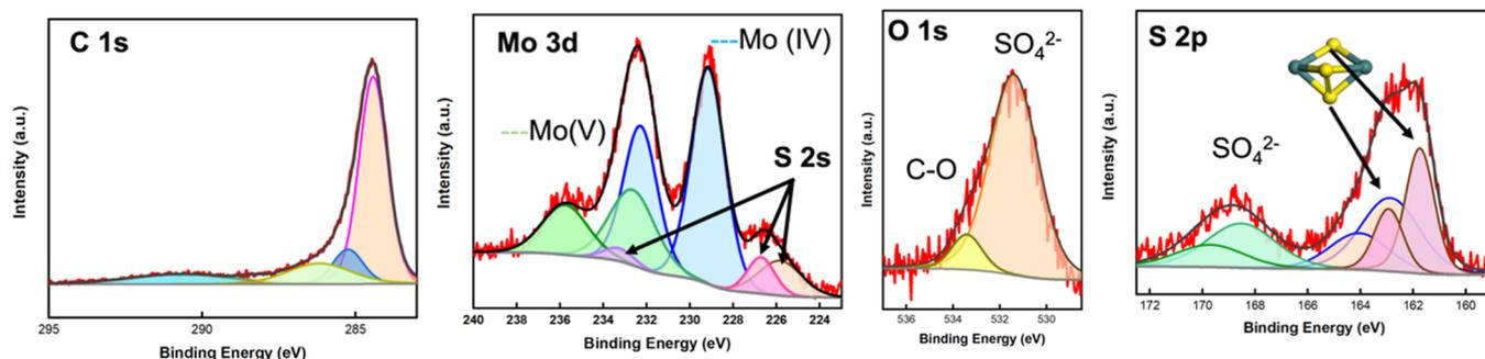
**Figure 5.** XPS spectra for the  $\text{MoS}_x\text{@MWCNTs}$ , (red) experimental data, (black) sum envelope, and doublet signals for Mo 3d and S 2p are indicated with the same color.
