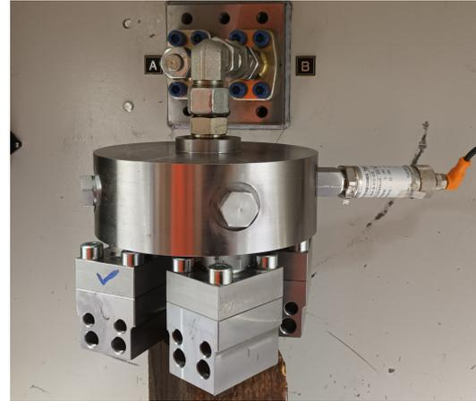
(b) Flow divider with four test specimens and a mounted pressure sensor.
