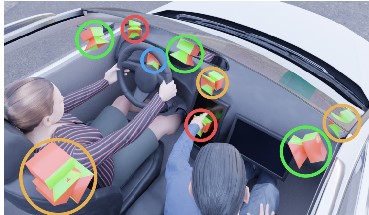
Figure 3.5: Overview of all camera positions evaluated on synthetic data rated from good (green) to unsuitable (red). The camera on the steering wheel column (blue) is only suitable to monitor the drivers head.
