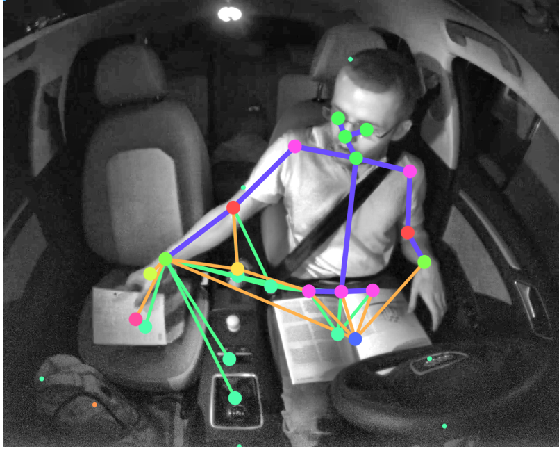
Figure 5.8: Reprojection of the 3D Dynamic Interaction Graph on a reference image for the activity fetching an object with body pose edges (blue), interior edges (orange) and object edges (green). The color of each point indicates its category.
