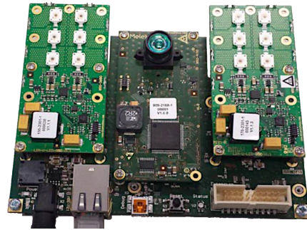
Figure 3.2: Specifications of the Melexis ToF Evaluation Kit.
