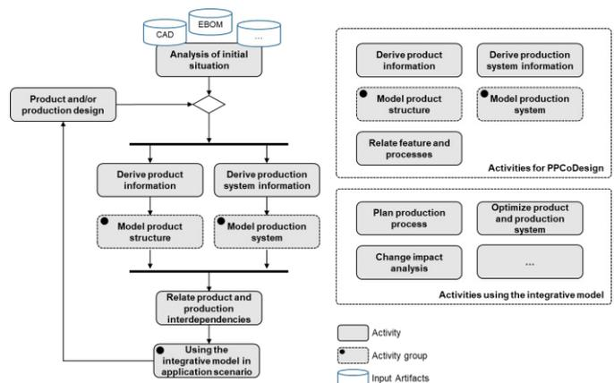
Fig. 3. Method for Developing Product-Production-Models.
