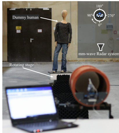
Figure 3.22: Setup for monostatic high-resolution RCS measurement of VRUs to extract their radar model (dummy human is placed on top of the rotating stage for extracting its scattering points) (Figure based on [1], ©IEEE).
