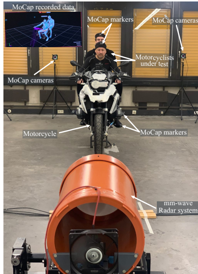
Figure 5.16: Setup for monostatic high-resolution RCS measurement to extract the range, velocity, and RCS information of different body parts of two motorcyclists in motion.
