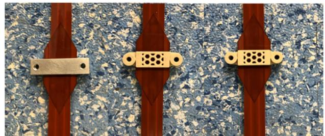
Fig. 4. Mechanical supports at 30 K and 80 K. The 30 K mechanical support (left) is made of aluminium and acts as a heat sink, while the 80 K mechanical supports (middle and right) are made of 3D-printed PEEK with a low thermal conductance.
