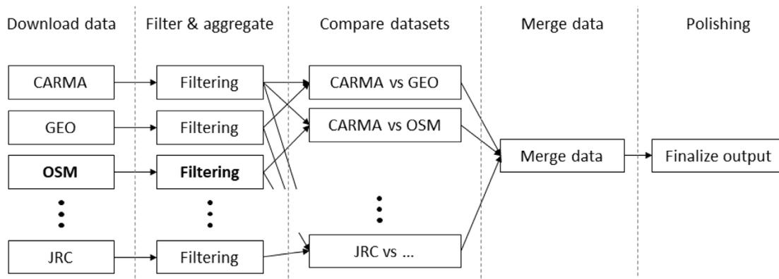
Fig. 4. Flowchart of the *powerplantmatching* procedure, including the novel OSM input (in bold) which was developed for PyPSA-Earth.
