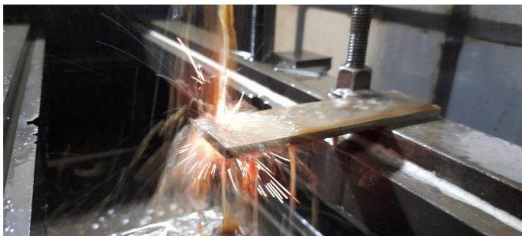
**Figure 3.** Experimental setup for wire EDM of stainless steel 304.
