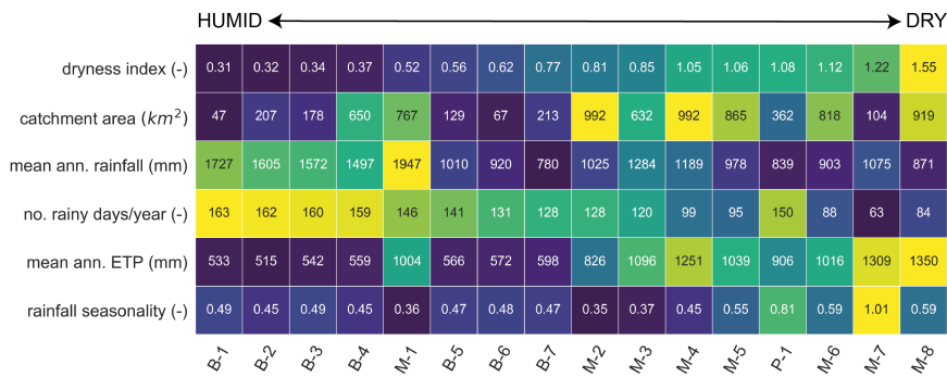
Figure 7.1: Overview over catchment and climate characteristics of the selected catchments (sorted by ascending dryness index). Color scale: yellow indicates high values, blue indicates low values, normalized to the range of each variable.
