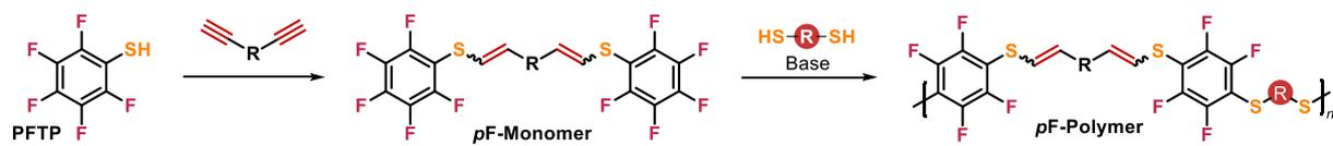
**Scheme 6.1:** Depiction of the general concept for the synthesis of a symmetrical monomer based on PFTP and dialkynes and subsequent polymerization via *para*-fluoro thiol reaction with dithiols.
