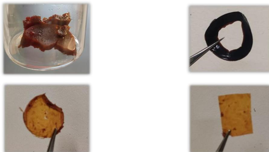
**Figure 4.2:** Photographs of selected crosslinked specimen from the reactions summarized in **Table 4.2**. *Top left:* Fully crosslinked material which took the shape of the reaction vessel. *Top right & bottom left:* Ring and circle shaped networks obtained during drying in vials. *Bottom right:* Rectangle cut from the circle (*bottom left*), evidencing the self-supporting nature of the crosslinked material.
