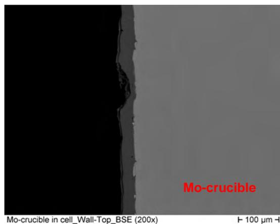
**Figure 5.48:** BSE image of cross-section of the upper region of side wall of Mo-crucible after cell operation.
