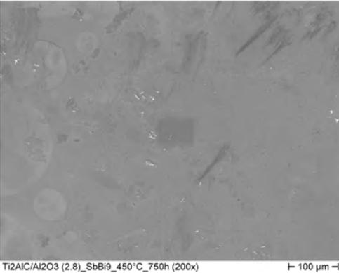
**Figure 4.54:** SE image of surface morphology of  $Ti_2AlC$  on  $Al_2O_3$ -substrate after 750 h exposure in liquid  $SbBi_9$  at 450 °C.
