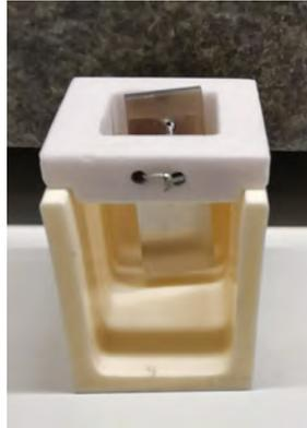
**Figure 4.16:** Cross-section of a sample holder ( $\text{Al}_2\text{O}_3$ -crucible with an  $\text{Al}_2\text{O}_3$ -holder on top) for corrosion tests for PCC materials at fully-charged state and a sample (fixed on  $\text{Al}_2\text{O}_3$ -holder by Mo-wires) inside.
