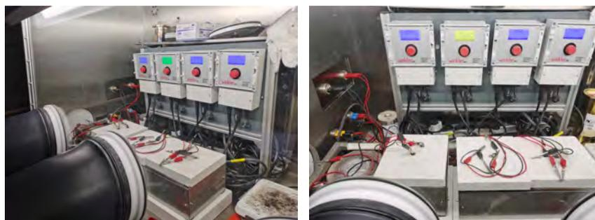
**Figure 5.4:** Heating sleeve and temperature regulator with alumina covers for cell testing.
