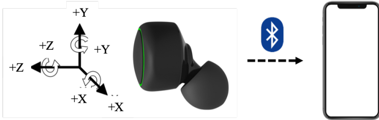
Figure 3.2.: The Nokia Bell Labs eSense earphones [235] connect via BLE to transfer gyroscope and accelerometer data to a smartphone app.
