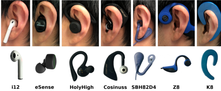
Figure 6.8.: Earables selected for the study, ranging from in-ear to ear-hooks.
