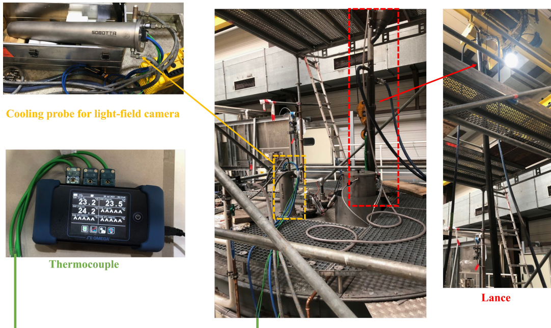
Figure 2.6.: Images of the experiments conducted in the combustion chamber. The plenoptic camera cooled by a cooling probe installed at the top of the combustion chamber is marked with a yellow dashed rectangle. The real-time temperature inside the cooling probe is measured and displayed by the thermocouple on the left side. A height-adjustable lance is marked with a red dashed rectangle.
