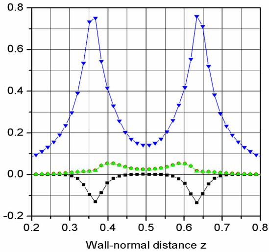
Figure 4. Wall-normal profiles of production term (dimension  $[m^2/s^3]$ ) at  $y=0.586$ . Exact term is denoted by  $\blacksquare$  and models from Table 1 by:  $\blacktriangle$  P1  $\bullet$  P2  $\blacktriangledown$  P3.
