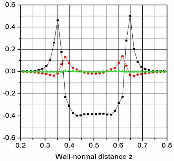
Figure 5. Wall-normal profiles of diffusion term (dimension  $[m^2/s^3]$ ) at  $y=0.586$ . Exact term is denoted by  $\blacksquare$  and models from Table 2 by:  $\bullet$  D1  $\blacktriangle$  D2.
