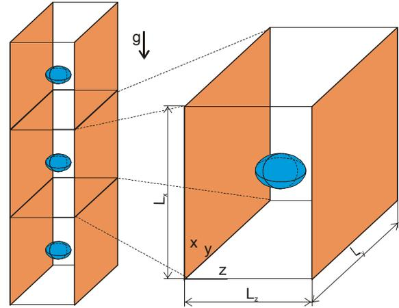
Figure 1. Geometry of computational domain.
