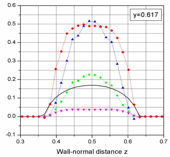
Figure 6. Wall-normal profiles of interfacial terms (dimension  $[m^2/s^3]$ ) at different span-wise positions,  $y$ .  $\bullet$  indicates exact term. Model assumptions listed in Table 3 are denoted as:  $\blacktriangledown$  Morel (1997)  $\blacktriangle$  Pflieger and Becker (2001)  $\blacklozenge$  Hill et al. (1995). The black solid line represents mean gas volumetric fraction.
