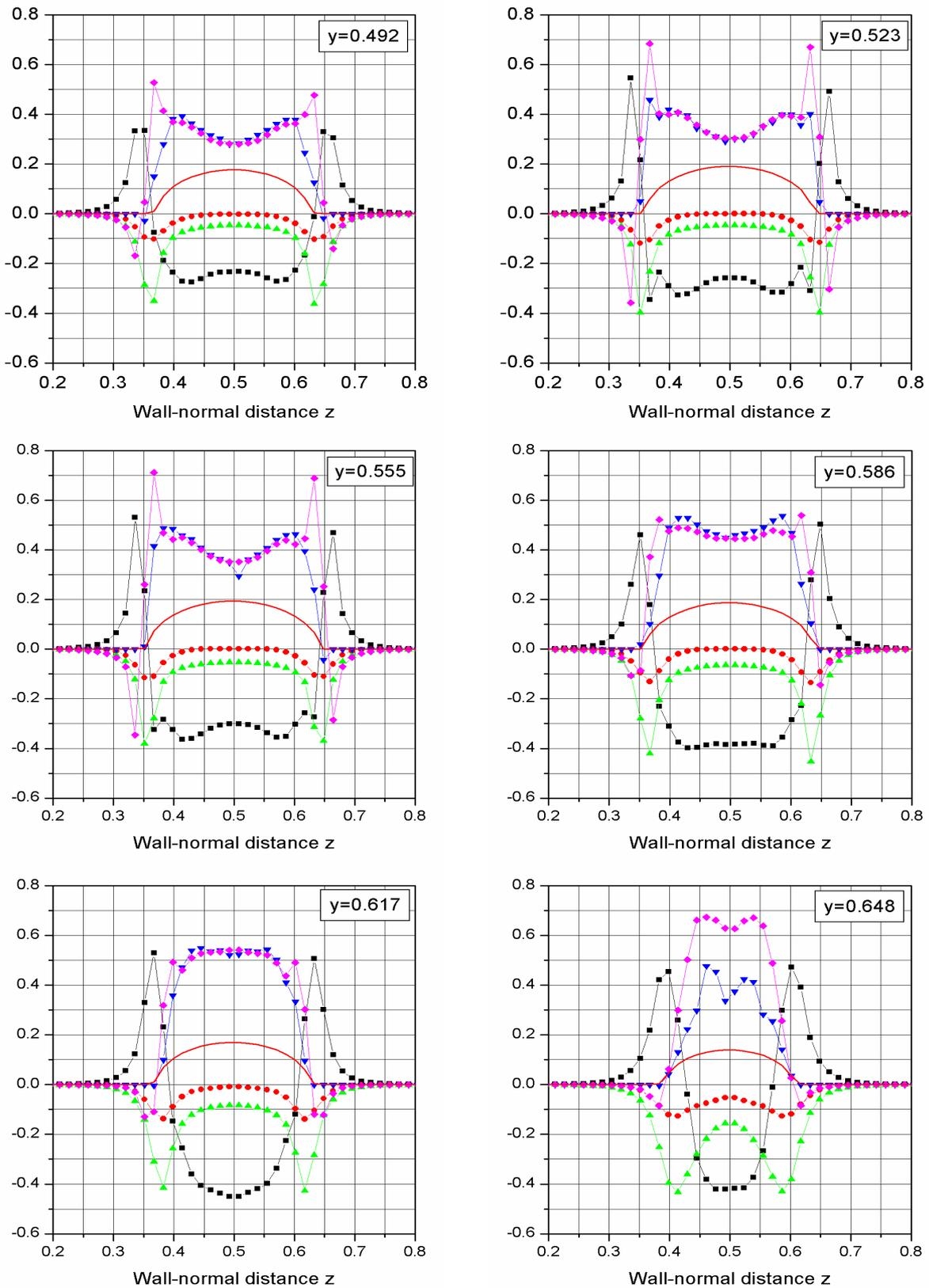
Figure 3. Wall-normal profiles of balance terms in equation (4) calculated for different span-wise positions. Legend: ■ diffusion, ● production, ▲ dissipation, ▼ interfacial terms calculated from equation (4) ◆ interfacial terms estimated from equation (14). Balance terms from  $k_L$  equation are displayed with dimension  $[m^2/s^3]$ . Mean value of gas phase volumetric fraction is represented by solid red line.
