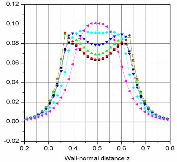
Figure 2. Wall-normal profiles of turbulence kinetic energy (displayed with dimension  $[m^2/s^2]$ ) for the following span-wise positions,  $y$ : ■ 0.492 ● 0.523 ▲ 0.555 ▼ 0.586 ◆ 0.617 ▲ 0.648.
