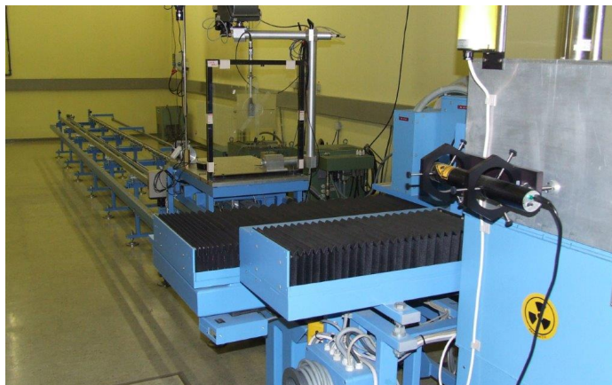
Figure 3.4 Irradiation bench for ^{137}\text{Cs} photons
