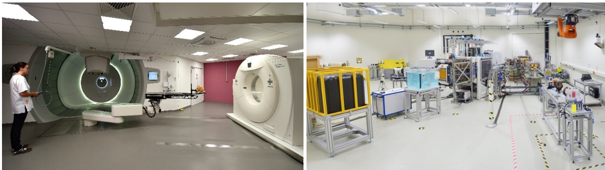
Figure 3.8 Picture of treatment room of the University Proton Therapy Dresden (left) and the experimental proton room with two horizontal beam lines (right).
