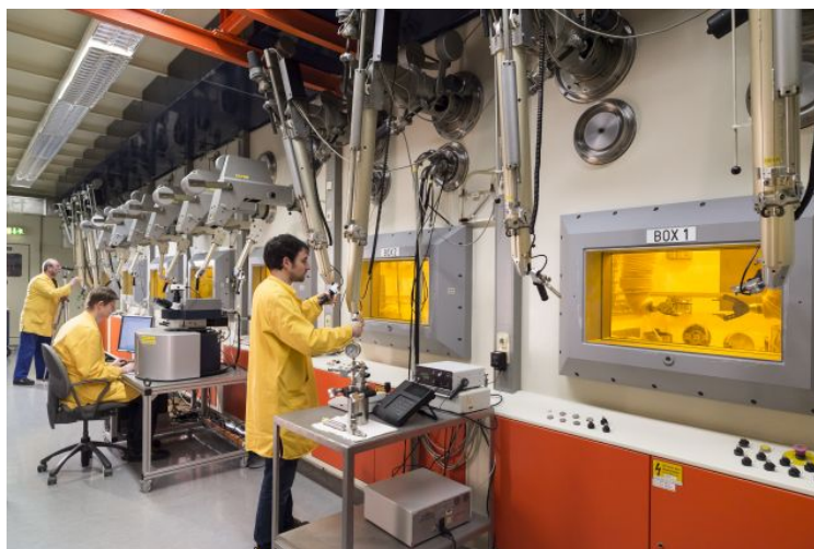
Figure 3.3 Infrastructure of the shielded box line/hot cells at INE
