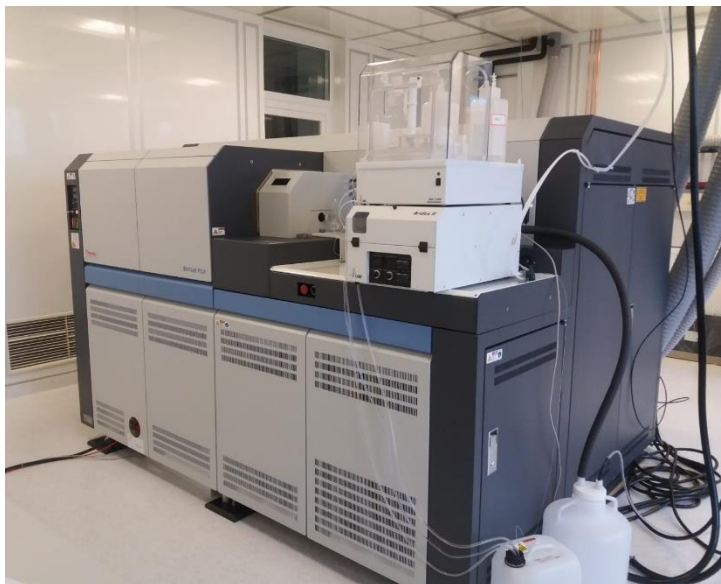
Figure A-7: Thermo Scientific Neptune MC-ICP-MS in the Soil Biogeochemistry laboratory of the KIT-Institute of Geography and Geoecology.
