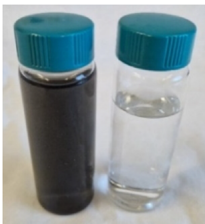
Figure 5. Reactor effluent sample taken without and with filter installed (experiment 1).
