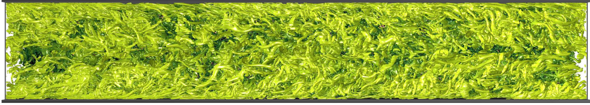
Figure 7.36: Visualisation of instantaneous vortex clusters in case DL500^{H2} ( t/T_b = 23 ) as seen from the top of the open duct. The structures were detected as connected regions for which the discriminant of the velocity gradient tensor, \mathcal{D} , is larger than 2% of its local r.m.s. value. In contrast to the extraction procedure outlined in the text, we here use for visualisation purposes only the instantaneous r.m.s. value \langle (\mathcal{D} - \langle \mathcal{D} \rangle_x)^2 \rangle_x^{1/2} rather than \mathcal{D}_{rms} , as statistics of \mathcal{D} have not been computed for the entire time series in this case. Colouring of the individual structures represents their distance to the bottom wall and thus the sediment bed, with brighter green clusters being located closer to the free surface than dark green objects. Flow is from left to right.
