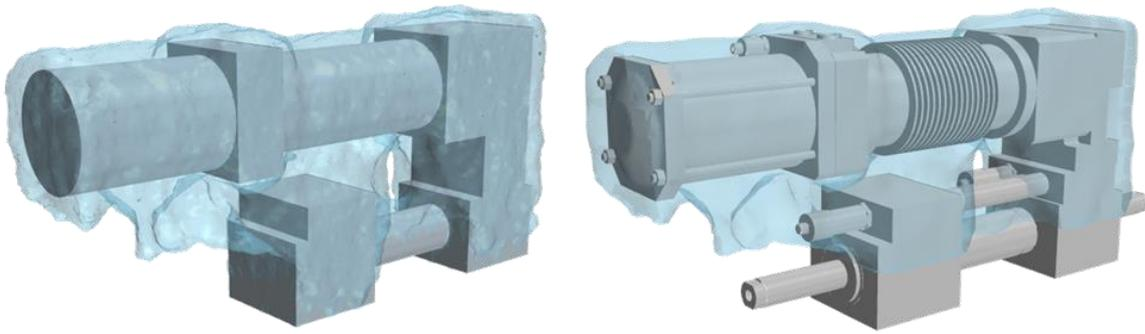
**Figure 5. Optimization result of the preliminary optimization (left) and remeshed optimization result transferred to the detailed simulation model (right).**
