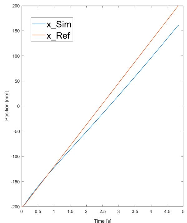
Fig. 6. Position of X-axis simulated (blue) and reference drive (orange).
