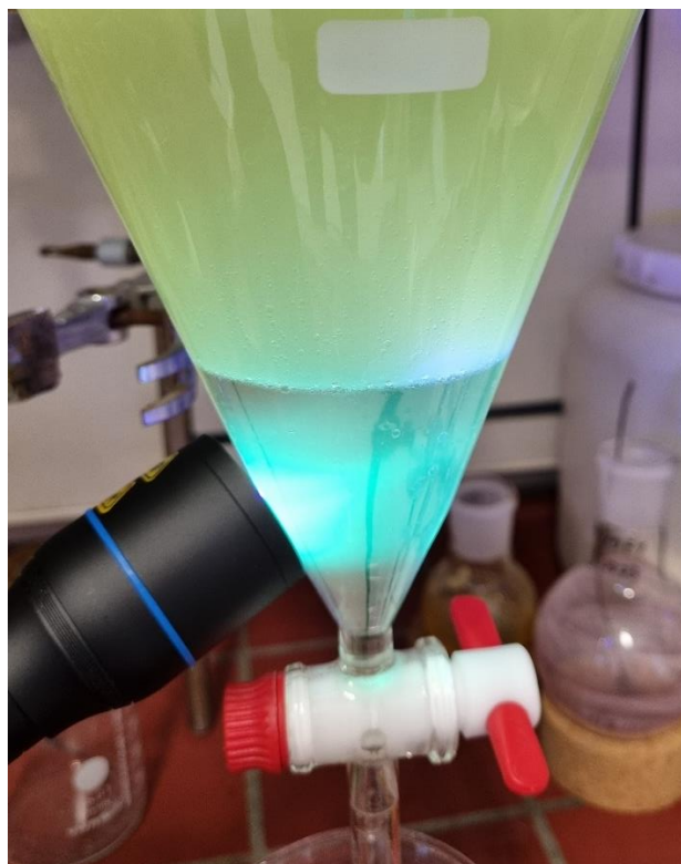
Figure 30. Successful extraction of the fluorinated HINA derivatives could be observed by irradiation with UV light.
