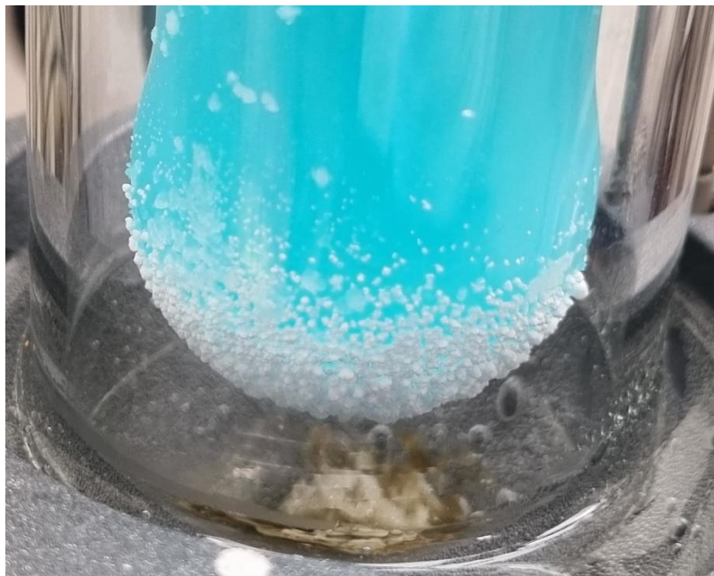
Figure 19. Sublimation of crude 38 in a sublimation apparatus under reduced pressure. The blue liquid is the cooling mixture being pumped through the apparatus.
