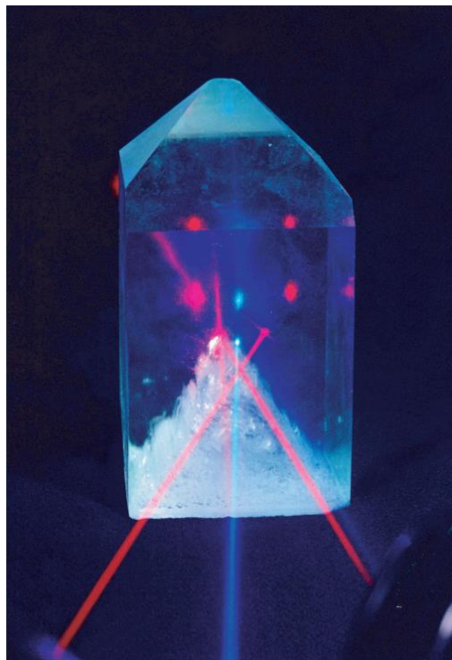
Figure 9. SHG process in an ammonium dihydrogen phosphate crystal. Reproduced from ref. [76] with permission from the Royal Society of Chemistry.
