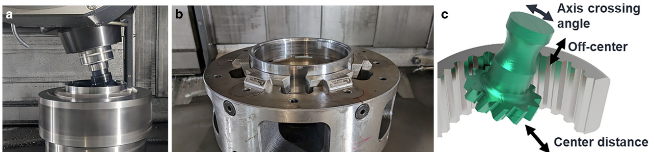
Fig. 7 (a) Process setup. (b) Six-bolt-chuck. (c) Degrees of freedom in gear skiving
