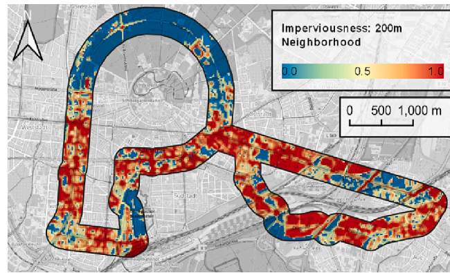
Fig. 7. Representation of the gray infrastructure in the 200 m neighborhood to the route by remotely-sensed imperviousness (European Union, 2018). This layer contains the sealing in the entire urban area in 20 m spatial resolution. (Basemap by OpenStreetMap).
