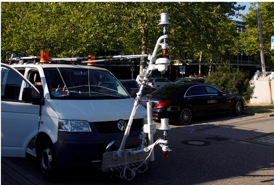
Fig. 2. Measurement vehicle of the German Meteorological Service to measure air temperature, relative humidity (at 0.7 m and 2.0 m height above ground level (AGL)), surface temperature and global radiation.
