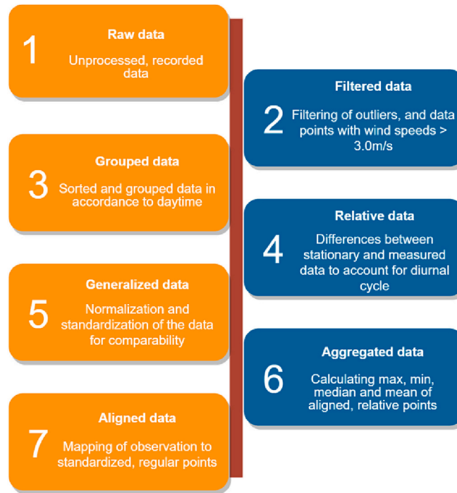
Fig. 3. The steps for preprocessing and preparation of recorded data for the Spatial Neighborhood Analysis.
