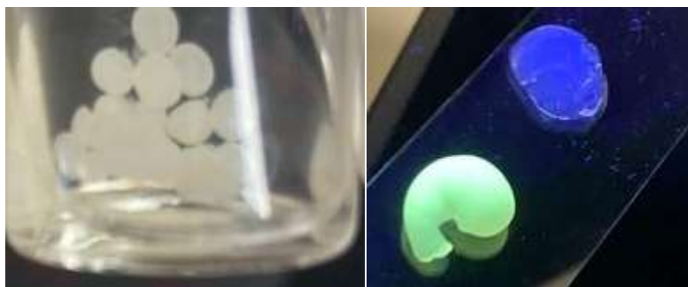
Figure 84. Left Alginate beads through ionic bonds with calcium and containing CAT- 23 as CAT Right: Alginate gel formed through ionic bonds with calcium and containing PS- 24 irradiated under UV light.
