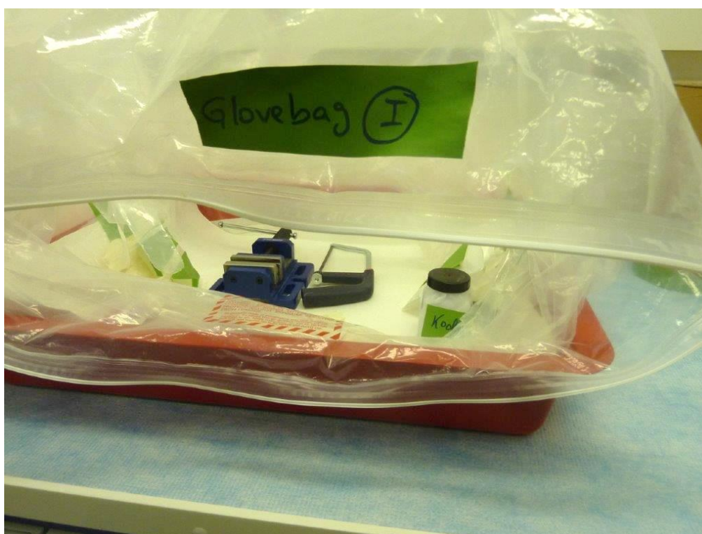
Fig. 31 Glove bag, equipped with handsaw, vise, and KODAN® tissues.
