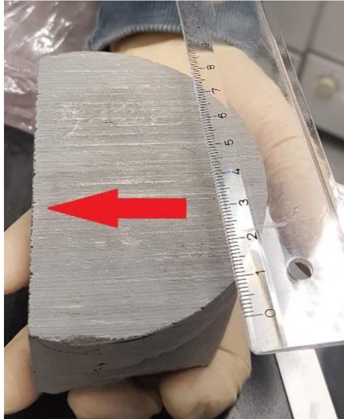
Fig. 21 Piece of OPA bore core BLT-14, red arrow indicating the orientation of bedding.
