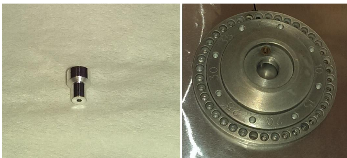
Fig. 17 Pictures of aluminum sample cathode (left) and sample wheel holding up to 40 sample cathodes (right).
