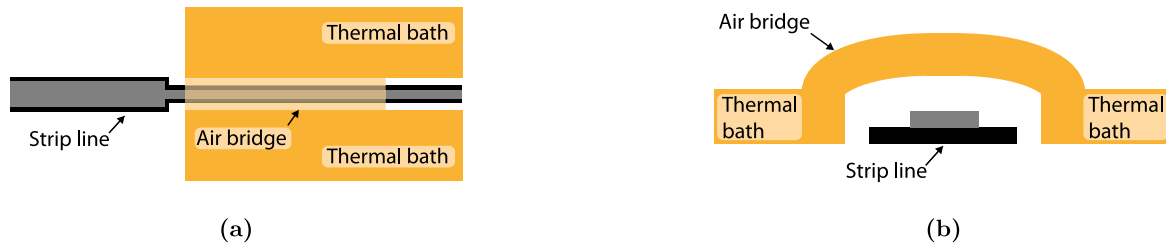
Fig. 5. Top (a) and side (b) views of the air bridge structure to connect consecutive thermal baths in the ECHO-100k design. The thermal baths are separated by niobium strip-lines (consisting of two overlapping niobium lines with isolation in between).
